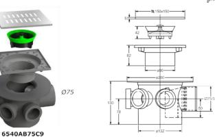
"Hellas" Floor gully with removable hydraulic siphon (water seal : 50 mm) Ø125 mm top female inlet. Gluable with PVC / ABS glue.
