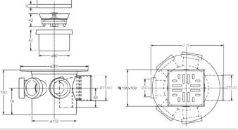
"Hellas" Floor gully with removable hydraulic siphon (water seal: 50 mm) and with non-return mechanical valve that prevents bad smell even in absence of water. Gluable with PVC / ABS glue.
