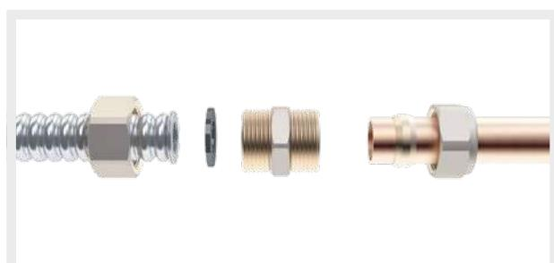
In the connection between PLT-CSST tubes or PLT-CSST tube with other copper tubes the tightness is assured through the use of a plane gasket (flanged tube) and on the other side through the compression of a brass ogive (for copper tube conform to EN 1057 R220 "annealed" or R250 "half hard", an additional reinforcement bush may be necessary).
