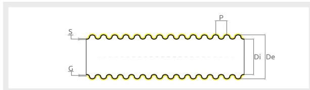
Di: Diametro interno / Internal diameter
