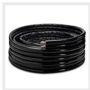
Mono Sun Set and Twin Solar Set lines are composed by PLT-CSST tube in AISI 304, thickness 0,3 mm with EDPM closed cell structure insulation coating and covered with mechanical ware and UV protective film.
