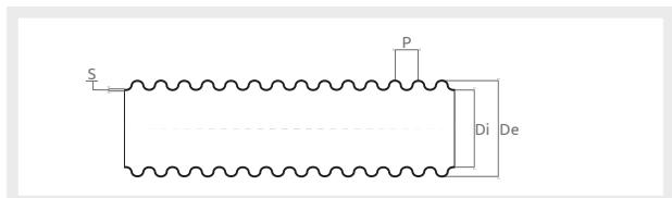
Di: Diametro interno / Internal diameter
