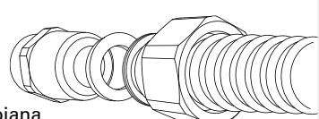
Using the fittings with tightness through plane gasket the PLT-CSST tube have to be previously flanged using the manual, semi-automated or automated flanging tools supplied by Eurotis:
