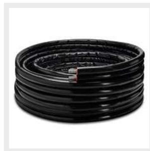
Solar Thin Power composed by PLT-CSST tube in AISI 304, thickness 0,3 mm, preinsulated with a special formulation of flexible expanded polyurethane that makes the tube suitable for continuous operative temperature up to 150°C.
