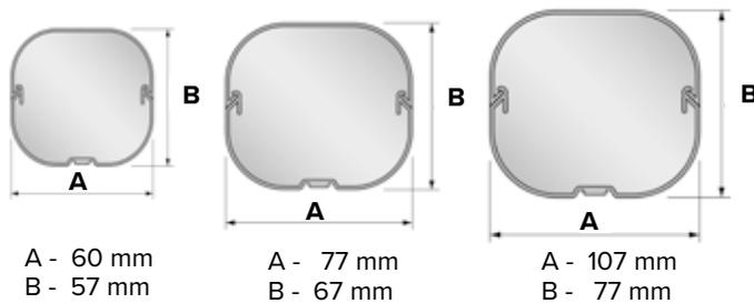
**CANALINA PER TUBI IN BARRE DA 2 METRI**
